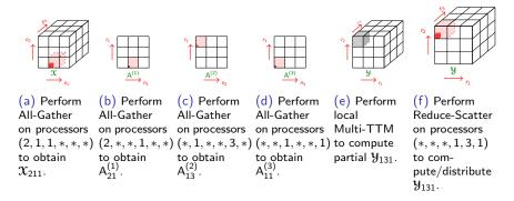
Steps of the algorithm for processor (2, 1, 1, 1, 3, 1), where  $p_1 = p_2 = p_3 = q_1 = q_2 = q_3 = 3$ . Highlighted areas correspond to the data blocks on which the processor is operating. The dark red highlighting represents the input/output data initially/finally owned by the processor, and the light red highlighting corresponds to received/sent data from/to other processors in All-Gather/Reduce-Scatter collectives to compute  $\mathcal{Y}_{131}$ .
