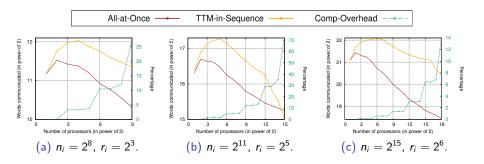
Communication cost comparison of all-at-once approach (the presented algorithm) and TTM-in-sequence approach (of TuckerMPI). *Comp-Overhead* shows the percentage of computational overhead of the all-at-once approach with respect to the TTM-in-sequence approach. Cost of an approach represents the minimum cost among all possible processor configurations.
